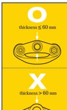
DeFender M1 fits most standard front forks. However, it will not fit forks with a crown thickness over 60 mm (2.36") and is not designed to be used with the 1.5" headset standard.
